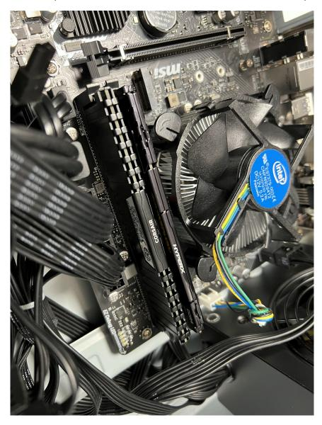
With the second stick of RAM now installed, I can install the GPU into the PCle  $16 \times 10^{-5}$  slot.
