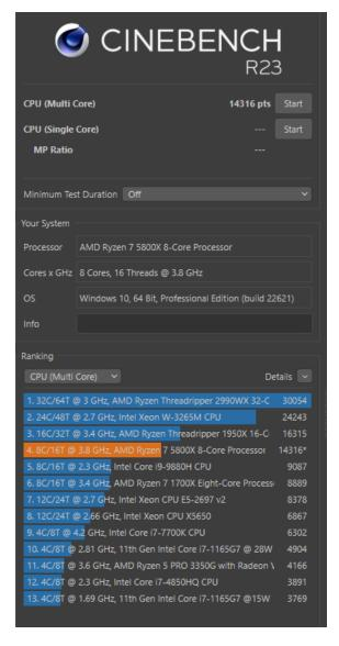
In this test, my PC scored 14,316. Compared to an Intel i9-9880H processor, mine was 1.58 times faster.
