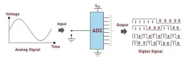
Figure 5: Basic example of how an analogue signal is converted to be digital electricalfundablog.com/analog-to-digital-converter-adc
