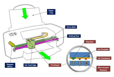
Figure 11: Internals of an Inkjet printer pintrest.com
