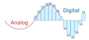
Figure 3: Basic example of an analogue signal being quantised into a digital signal mathsisfun.com
